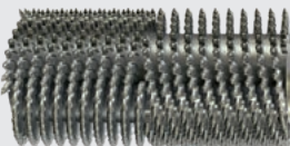
Micro-fine milling drum Milling width: 2,000 mm Milling depth: 0–30 mm Tool spacing: 6 x 2 mm
