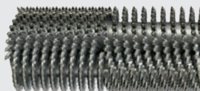
Micro-fine milling drum Milling width: 2,000 mm Milling depth: 0–30 mm Tool spacing: 6 x 2 mm
