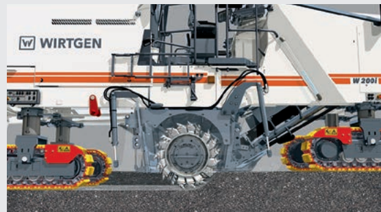
4 | The milling machine mills at full working depth right from the first metre
