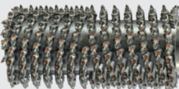
Fine milling drum Milling width: 2,000 mm Milling depth: 0–100 mm Tool spacing: 8 mm
