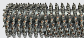
Fine milling drum Milling width: 2,000 mm Milling depth: 0–100 mm Tool spacing: 8 mm
