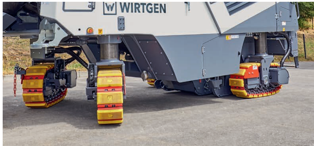
Impressive steering angle for use on narrow job sites.
