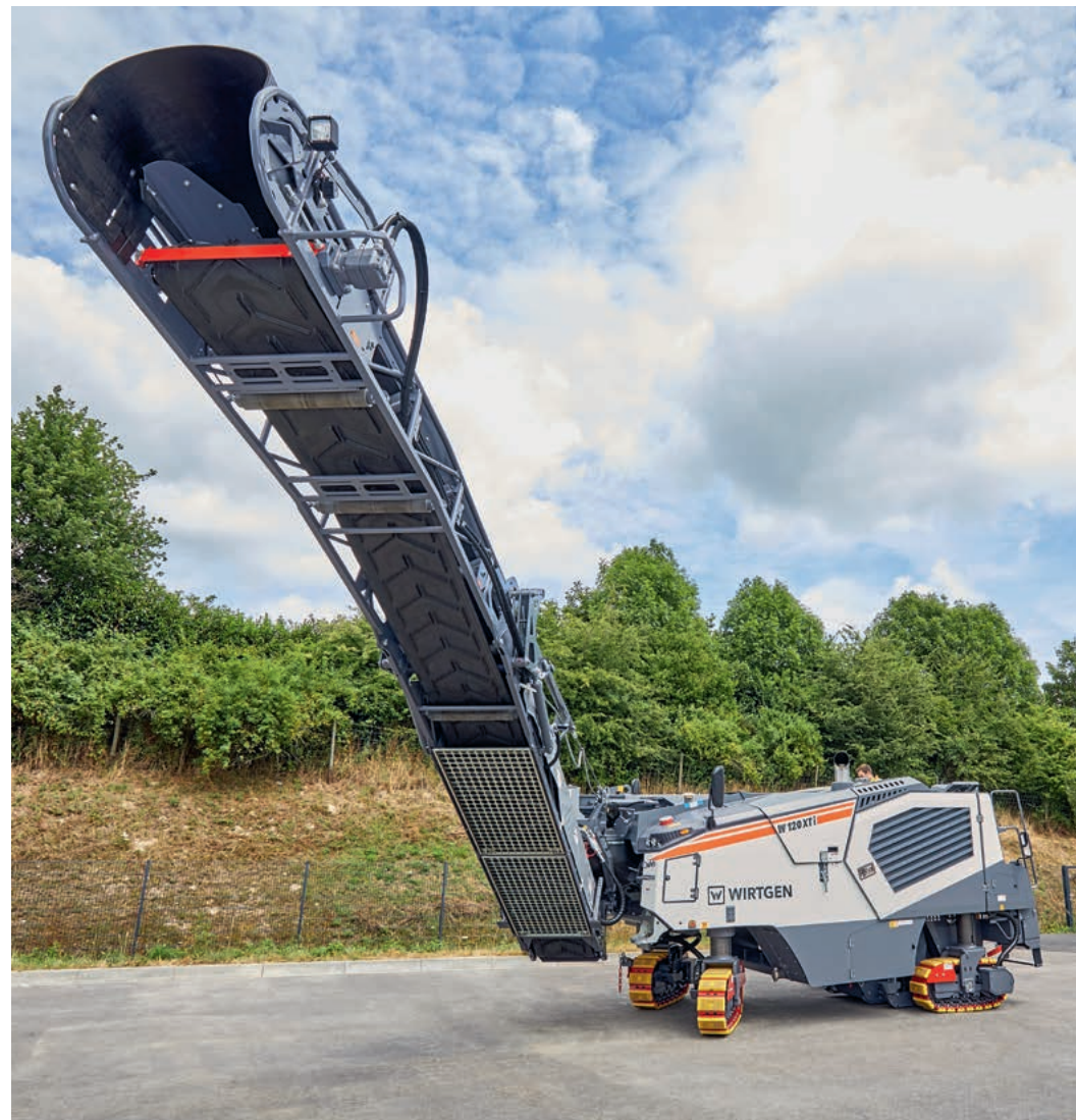
The discharge conveyor has a large swing range.
