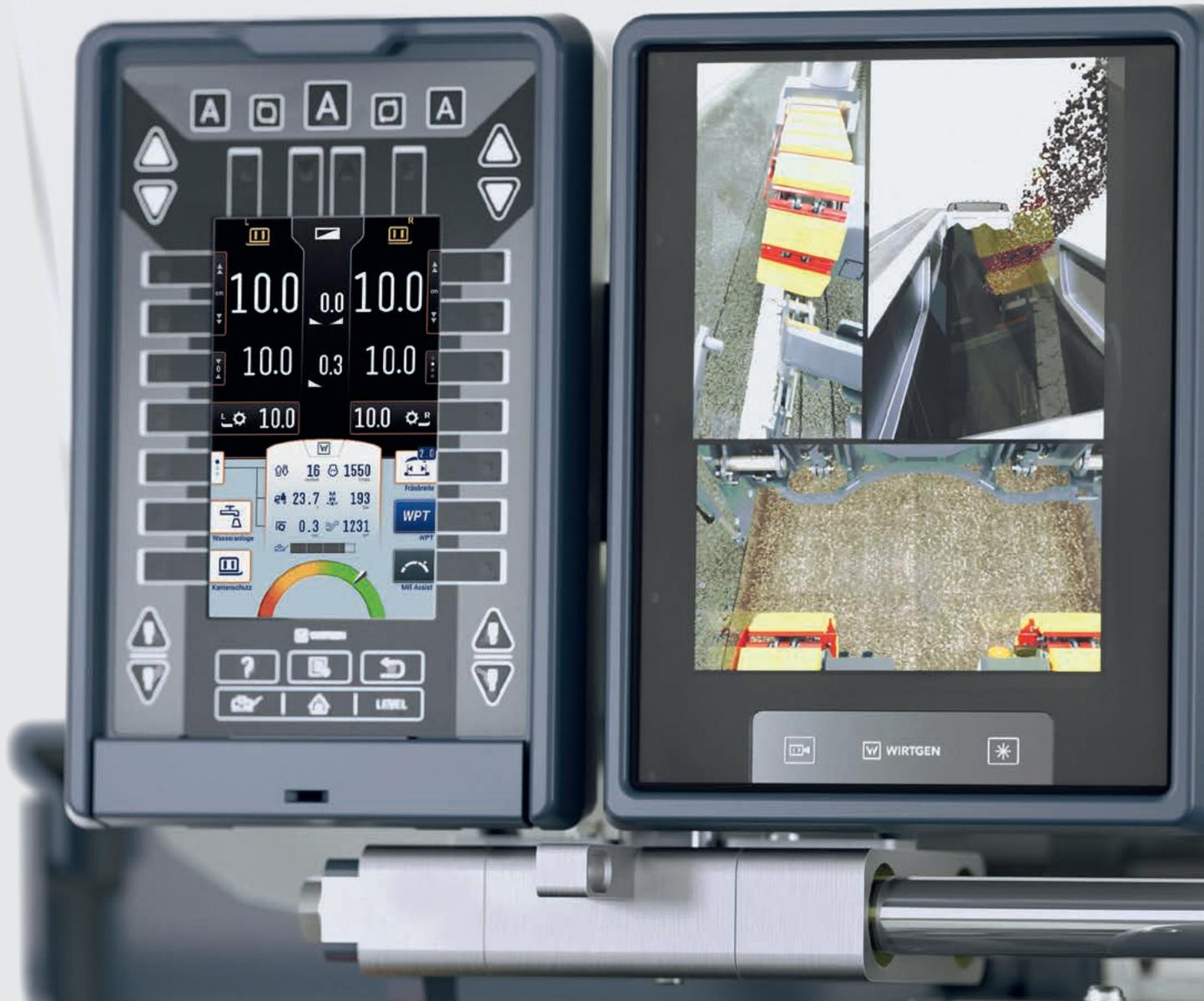
2 | Control panel for operating functions performed by ground crew.
