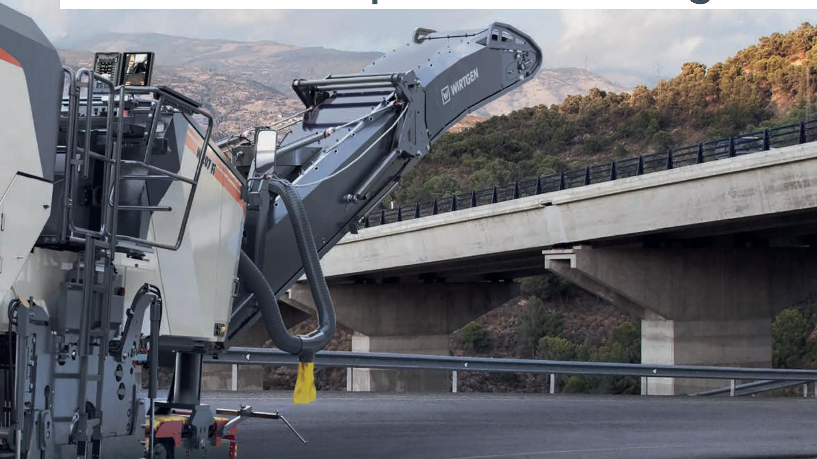
The easy-to-operate, powerful cold milling machine caters to a wide range of applications from surface course rehabilitation via pavement removal at full depth all the way to fine milling operations.
