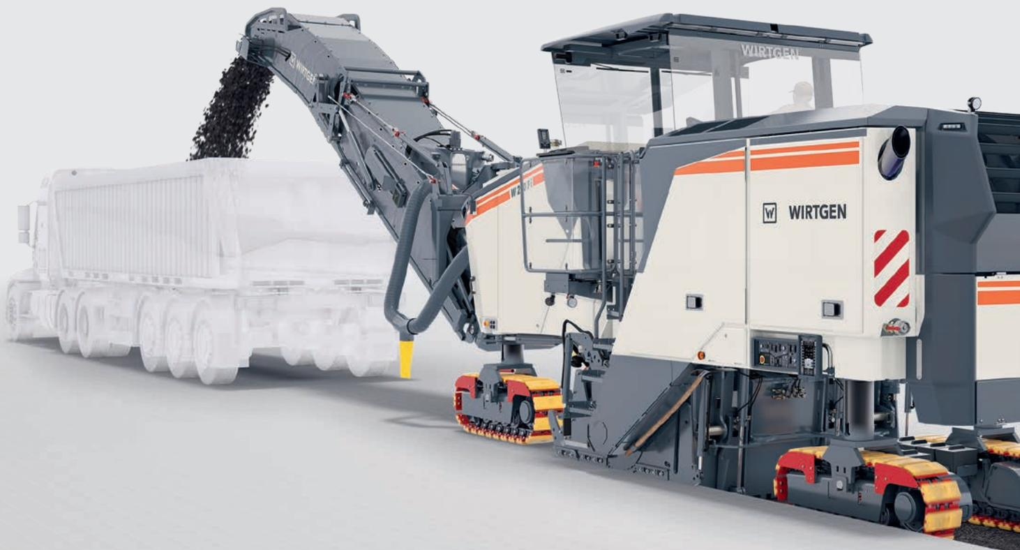
1 | Large slewing range of the discharge conveyor.
