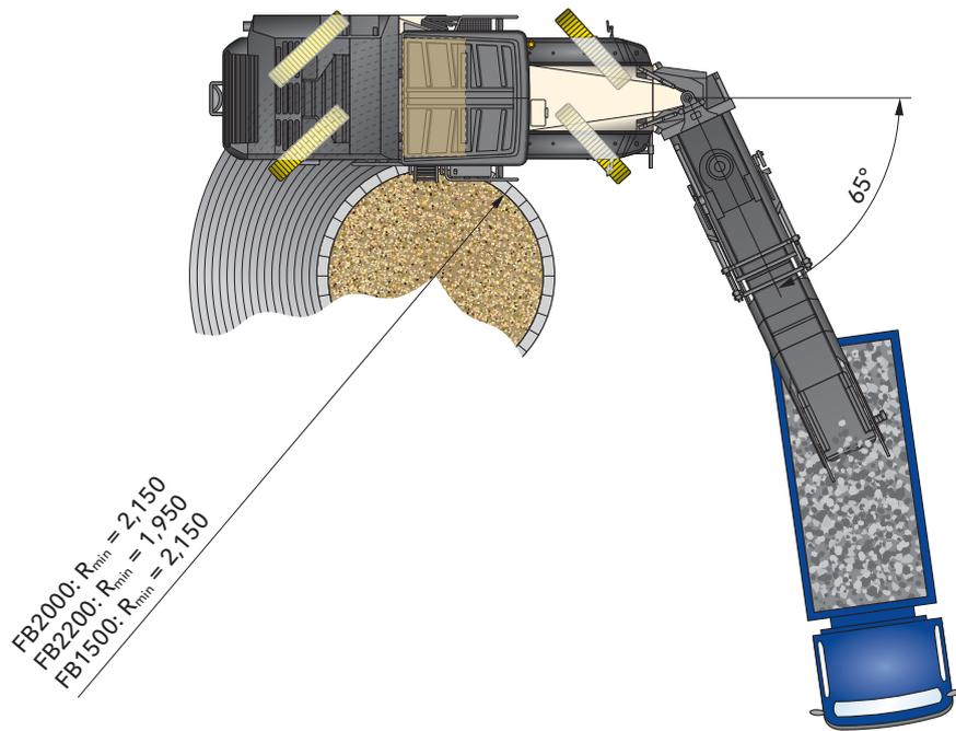
Milling radius, milling depth 150 mm, dimensions in mm
