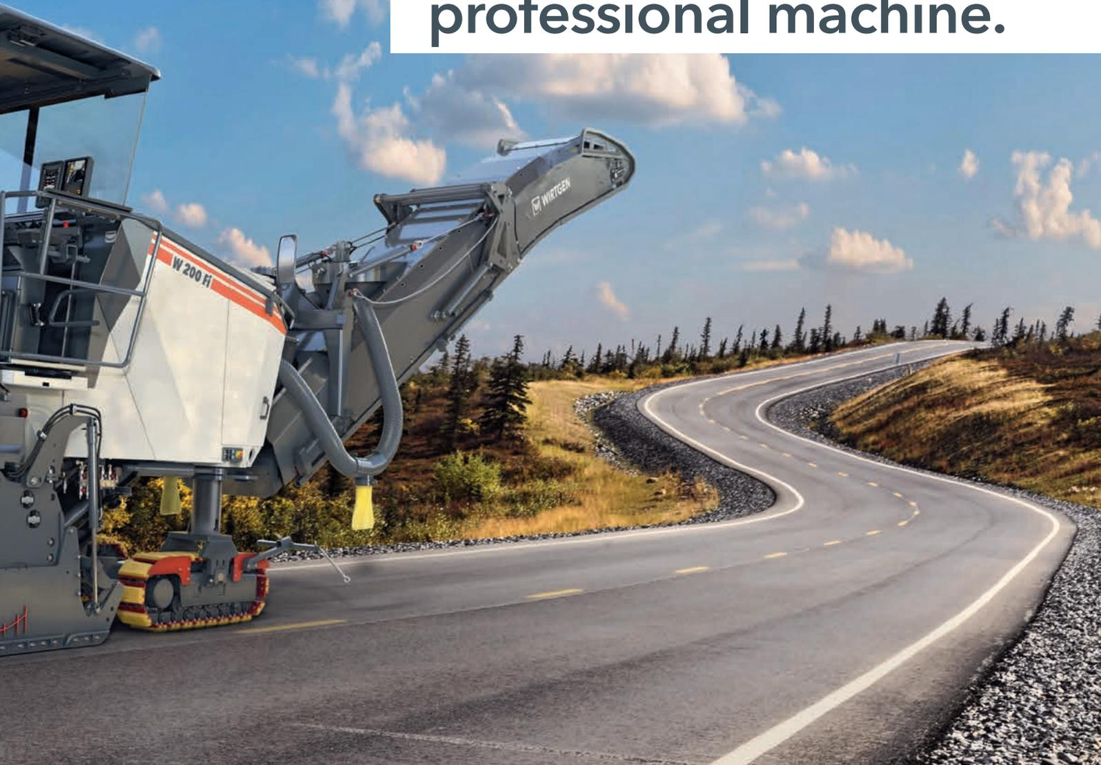
The easy-to-operate, compact cold milling machine caters to a wide range of applications from surface course rehabilitation via pavement removal at full depth all the way to fine milling operations.
